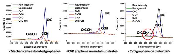
XPS analyses on the large-scale graphene films grown by CVD after each step. (a) A mechanically exfoliated graphene film on a silicon dioxide substrate for a reference. (b) A monolayer graphene grown by CVD on a Cu substrate and (c) After the transfer to a dielectric substrate.
