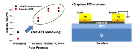
Electrical properties of the transferred graphene after the post annealing process. (a) Mobility variation using a back-gate transistor and the hall-effect measurement, and (b) FET structure using mobility measurement.
